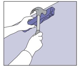
**9** Use a wood block wrapped in a soft cloth to work across the surface of each panel, tapping the block gently with a hammer to ensure the adhesive on all battens makes contact with the panel, particularly around the edges.
