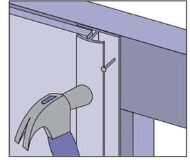
**10** Allow for a 3mm expansion gap on each side of the next joiner and nail or staple the joiner to the frame.
