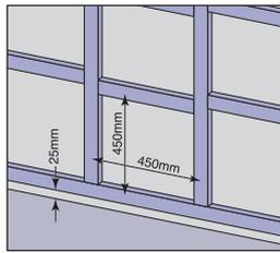
**1** We recommend that panels be fixed to a framework of timber battens 50mm x 25mm in size with a maximum spacing of 450mm between the vertical and horizontal battens. Ensure the lowest point of the frame is at least 25mm above the floor or shower base. Where two panels are joined together, place a timber batten behind the join and ensure the timber framework provides a flat surface.
