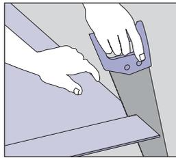
**2** When cutting straight lines use a fine tooth handsaw and always cut with the panel face up. If using a fine tipped tungsten machine saw ensure the panel is face down. Sand or hand plane cut edges to achieve a smooth finish. Use a fine toothed hacksaw to cut your colour-matched joiners to size.
